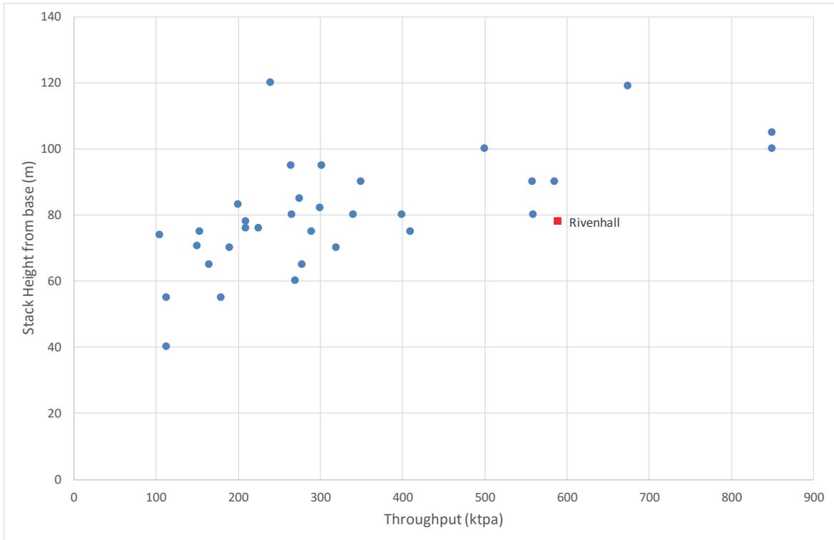
Figure 5 – Total Stack Height (physical length) against Throughput
